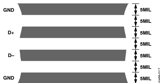
Figure 22. Typical Arrangement of Signal Tracks
